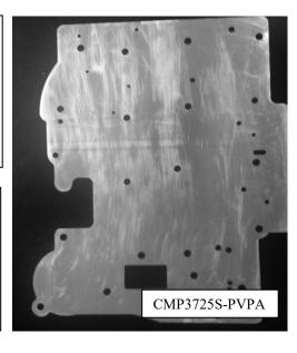
STEP 10: Start all of the valve body bolts before tightening to 110 in. lbs.
