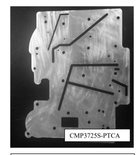
INSTALL A TRANSFER PLATE GASKET W/ ORANGE STRIPE ON BOTH SIDES OF THIS PLATE
