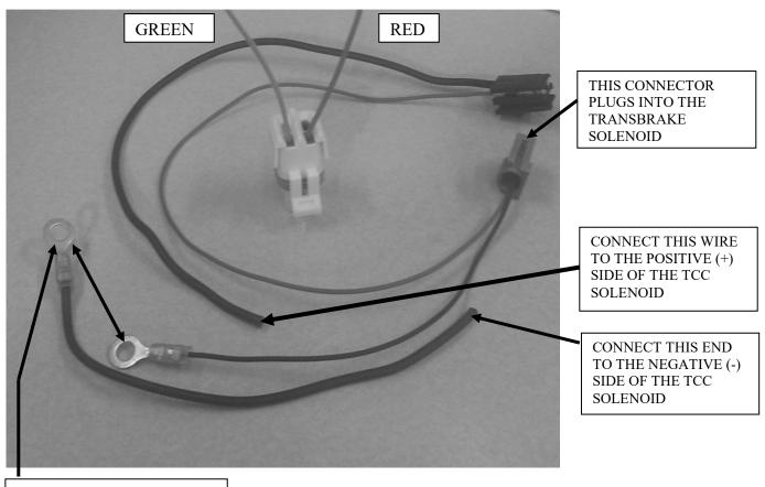
BOLT THESE TWO WIRES TO A SUITABLE PLACE ON THE VALVE BODY USING VALVE BODY BOLTS
