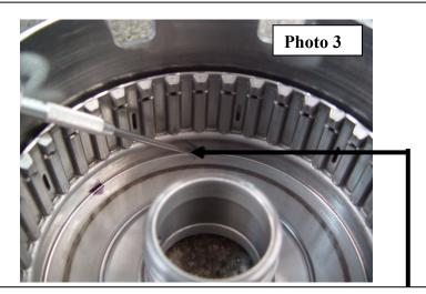
Drill a 1/16" hole approximately at a 45 degree angle at this location. Make sure the hole is drilled completely through the drum.
