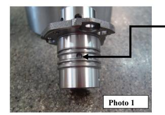
This hole in the stator tube must measure at least 0.215" or the stator tube must be replaced with a new stator tube TCI 373380.
