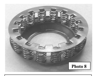
After the new springs are installed, install the spring stand as shown.
