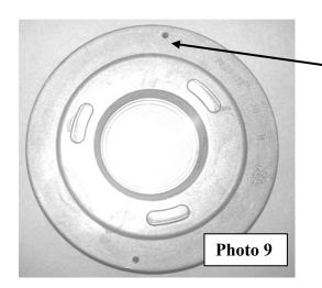
Install the set screw in the open bleed hole in the piston. Make sure the set screw is below the surface of the piston.
