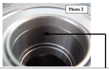
This hole in the reverse input drum must be a large square hole or the drum will need to be replaced. TCI 375560
